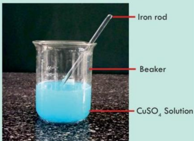
Figure 1.5 Reaction between iron and copper (II) sulphate.
