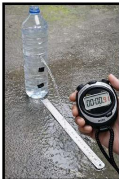
Gambar 2. Percobaan Teorema Torricelli Sumber: https://pin.it/4s7oDPwxA
