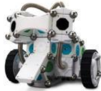
4. ModularRobotics/power/rechargeable LiPo battery
