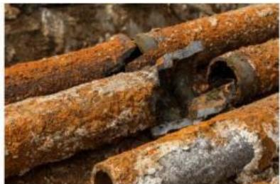
Rusting is actually a type of combustion reaction, similar to what happens with fire. When iron is in contact with oxygen, it reacts and forms rust. Unlike fire, though, this reaction happens much more slowly and without a flame.
