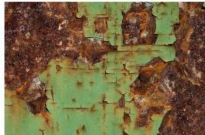
Rusting occurs when iron or iron-based metals, like steel, begin to corrode. The surface of iron corrodes first when exposed to oxygen and water, and over time, any piece of iron will turn entirely into rust and break down.
