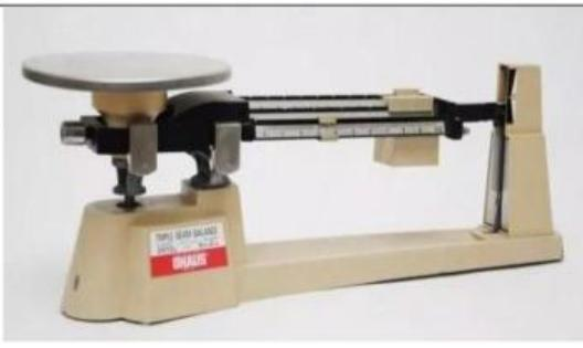
A triple beam balance scale is shown against a white background. It has a wooden base, a central vertical beam with weights, and a horizontal beam with a hanging weight pan. The base has a red label that reads "TRIPLE BEAM BALANCE" and "DRALIS". |  |  |
