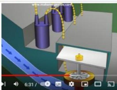
And inside the **generator**, **there is** a large \_\_\_\_\_ in the **coil** of **copper wire**. When this \_\_\_\_\_ **rotates** inside the **coil of wire** **electricity is produced**.
