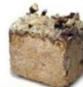
Fungi form mycelium, a network of very thin fibers that, when mixed with chopped up corn husks, produce a building material which is super strong, as well as water, mold and fire resistant.
