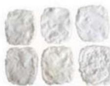
Seawater is separated into salt and freshwater, from which the salt is packed into moulds, dried and used for construction.
