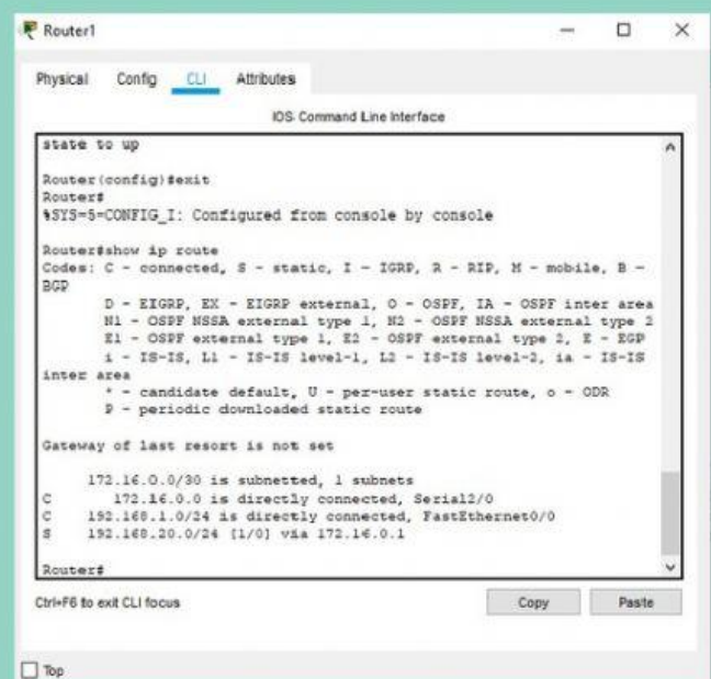
Gambar 13. Pengecekan Tabel Routing Router1
