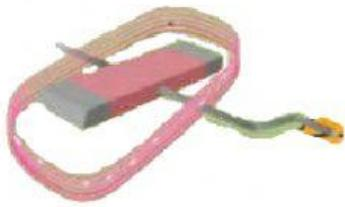
This is a **coil of wire** and **magnet mounted** on a **shaft** (eje). What it **is used** for? It **is used** to produce **electricity**. But how? If we **spin** a **magnet** around with-in (dentro de) a **coil of wire** **electricity is produced** in the **wire**. Oh, it is so simple! All we **need** to **have** is a **coil of wire** and a **magnet** to **make** **electricity**. And just **spin** the **magnet** with-in the **coil**. This process **is known** as **electromagnetic induction**.
