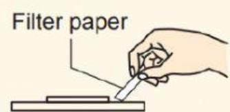
Absorb excess methylene blue solution
