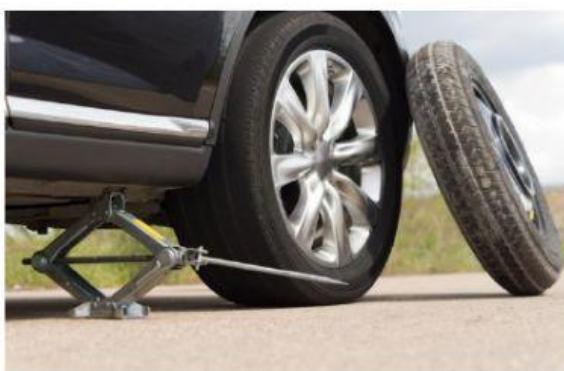
4. Remove the lug nuts that you loosened prior to using the jack by using the lug wrench.
