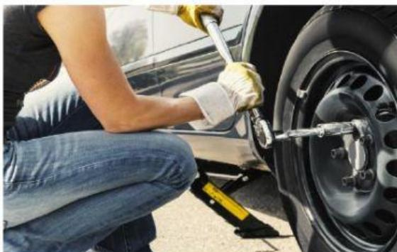
3. Use the jack to lift the wheel off of the ground.
