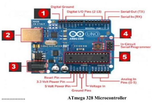
External power supply **USB** plug Analog reference pin Reset button
