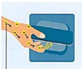
3. When you touch the metallic handle, the electrons can flow into it, giving you a shock.
