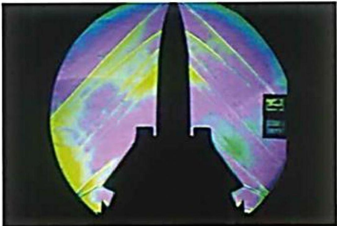
▲ **SCHLIEREN** *Schlieren photos use coloured lines to reveal invisible air moving around things. They are used to design more efficient shapes for aeroplanes and spacecraft.*
