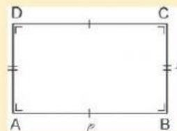
$$\begin{aligned}K &= p + l + p + l \\K &= (2 \times p) + (2 \times l) \\K &= 2 \times (p + l)\end{aligned}$$
