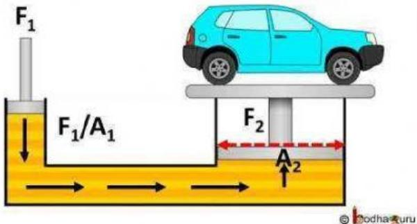
A hydraulic lift is used to lift a heavy machine that is pushing down on a  $2.8 \text{ m}^2$  platform with a force of 3,700 N. what force must be exerted on a  $0.072 \text{ m}^2$  piston to lift the heavy machine?
