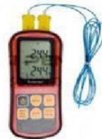
Gambar 5. Termometer termokopel
