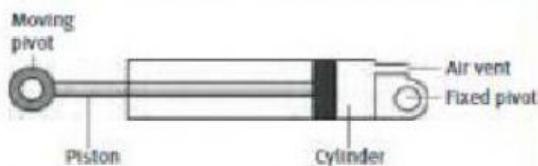
2 A picture of train doors is shown below. The doors of trains and buses work with pneumatic systems because the doors are light and have to open wide. Draw a system diagram of the two cylinders which will increase distance movement of the doors.
