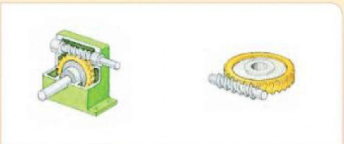
FIGURE 30 Worm gears are used in many everyday appliances
