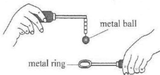
At room temperature the ball is able to pass through the ring.
