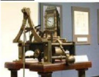
Double three-legged gravity escapement
