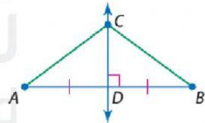
Line segment AC = line segment BC because CD is a perpendicular bisector.
