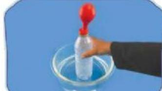
Immerse the plastic bottle into the glass container filled with hot water
