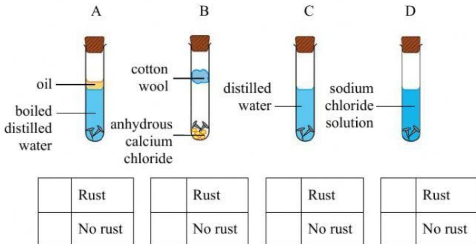
The nails in test tube \_\_\_\_\_ will be most heavily rusted.
