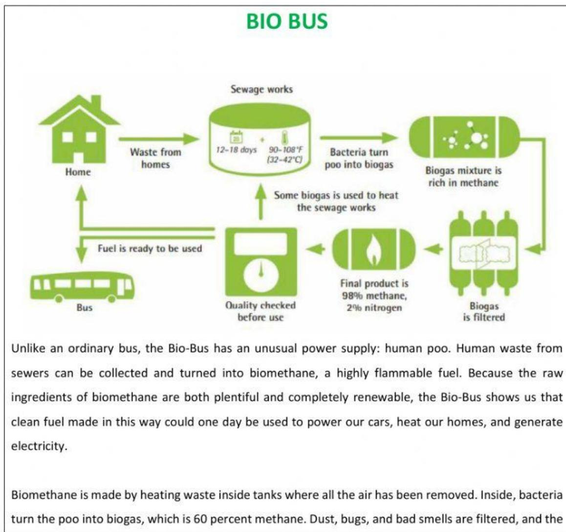
biogas is then refined, so it is 98 percent methane, which can be used as fuel for vehicles, or even supplied to homes.
